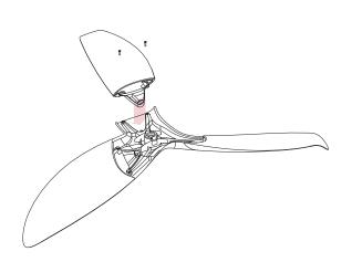
Place the Hub Upper onto a clean working area. Line-up the two mounting holes in the Fan Blade with the 2 holes in the Hub Upper.
