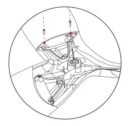
Fix the 3 Fan Blades tight and firm using 2 Hub screws for each Blade.
