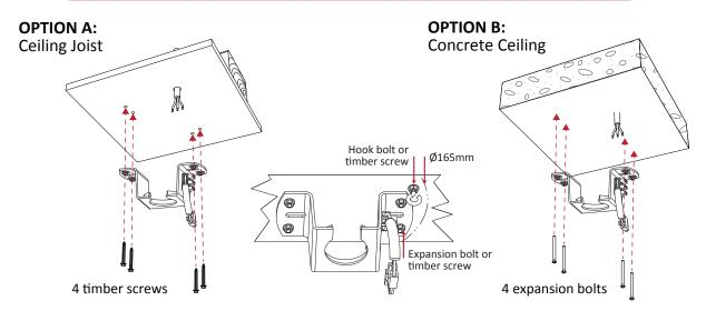
Install hanger bracket to ceiling joist or concrete ceiling using a minimum of (4) bolts/ screws as provided. Ensure ceiling joists are sound and of adequate size and strength to support a 32Kg (70lbs) load. If a timber frame is to be added it must be securely nailed or screwed between two beams. Mount the hook bolt / timber screws for the safety cable within the motor housing opening, approx Ø165mm from the centre of the hanger bracket.
